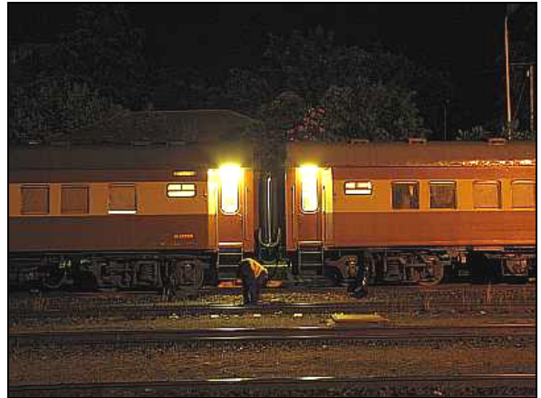
NT02 – Fred Sewell did a remarkable job on the lights. Many were repaired and many others were converted from inverter type systems to straight alternating current mains. But the outdoor vestibule lights are generally the most unreliable lights on the coaches due to exposure. The entire train had retained a full set of working vestibule lights by the time it had gotten to Ficksburg and in the rain too!
