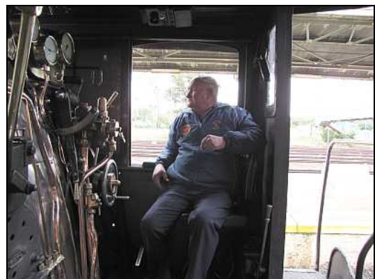
ST22 – Oom Attie finally comes on duty after working with the service team and assisting the trainee Train Manager. Attie does easily 85% of the Train Manager duties and hardly gets to drive these days. Notice that the duplex gauge at the top left is indicating vacuum on both sides, but you can see the vacuum ejector is isolated by the downward pointing lever just above the reverser's wheel. The electric locomotives are creating and controlling the vacuum. However, the pilot loco driver can still apply and release the brakes if he needs to in an emergency.
