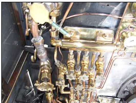
ST21 – I fired twice by hand – the first time upon departure with just a few spread-out scoops and lots of blower to reduce smoke in the station area. But I would have to face these controls for the journey as the 25NC doesn't steam well under load with a half loaded fire bed. For loco minding and pilot firing, you can get away with it but you have to consider what the crews need when shunting under our own power at the end of the pilot run.
