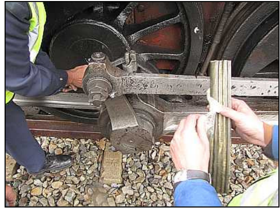
ST13 – Oh good! The grease sticks have arrived ... let the greasing commence. Piet is greasing the crankpin journal on the main driver. Dawie unwraps the long, firm plasticine-like sticks. As the weather is cold, they are harder than usual and are not very sticky – so they don't need to be lubricated with water to be handled. The bearings are warm enough to melt the grease within their working clearances.
