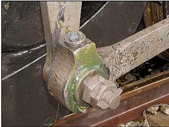
ST14 - This eccentric crank bearing on the 12AR was running hot and received an extra generous helping of soothing valve oil in an attempt to ease it up. The issue turned out to be clearances being slightly too tight on the Vesconite bushing. On this long distance run we had a longer time for the heat to build up compared to our normal day trips. After this check and receiving extra lubrication on the outbound trip, the bushing settled into service with no further problems.
