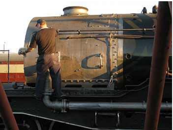
FP17 - Driver Chris Saayman stands astride the steam pipe that feeds the rear cylinders, while shaking out some waste. Chris was unable to reach a hard to service oil pot feeding a swivel pad, right in the corner of the smoke box and had to climb up to get in there. It was cleaned and serviced on the spot. (LG)
