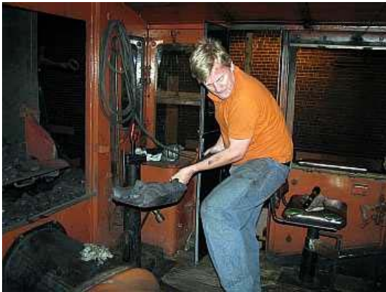
FP07 - The coal shovel two step - yeah, that's me discovering that this locomotive definitely ISN'T laid out for convenient hand firing with a long cab, an obstructive stoker tunnel, very low firebox doors and a high narrow hinged coal scuttle visible center left..
