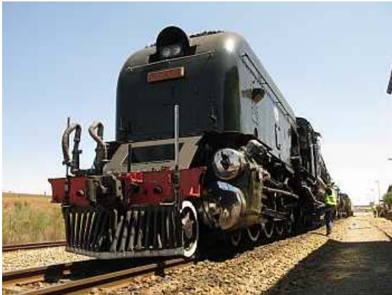
FP35 - Coach Controller Michelle Coetzee is just mounting the steps as the crew settle for the afternoon. The low angle shots emphasises the large scale of this "medium" gauge locomotive. Our country's 3ft6in "Cape Gauge" is narrow by the world's standards. (LG)
