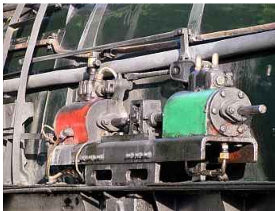
FP02 - The (slightly scruffy) Hadfield Reverser. On the Garratt it is back-to-front with the Lock Cylinder (Green) facing forward and the Actuator Cylinder (Red) facing the cab. Between the cylinders, notice the ingenious scotch-yoke arrangement that operates the drop-lever that, in turn operates the full-lengthed tubular actuating rod that runs alongside the massive boiler frames. (PA)
