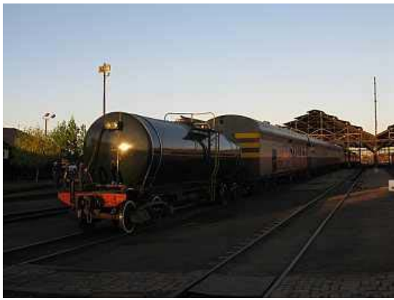
FP15 - Lyndie Lou's matching water tanker, also painted in dark Brunswick Green, catches the low morning sun as just-arrived coaching crew walk in from the new Reefsteamers car park. This tanker had a good helping of rust within the 33 000 litres of water and that rust would cause water feed problems on the way home. But for now, all is innocence. (LG)
