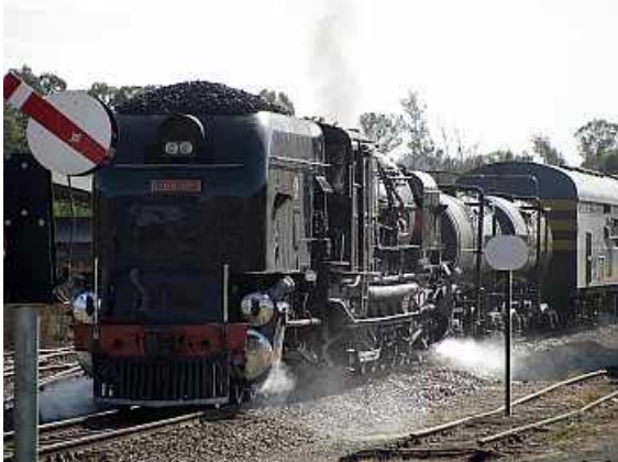
FP41 - Running bunker-first and with the cylinder cocks open, the coke all drunk and the braai meats masticated, it was time to leave. We were delayed waiting for a passing diesel hauled container train, which diesel-chugged us right back into the present. The two pivoting engine units of a Garratt are independent but notice how they are almost perfectly 180 degrees out of synch here. (PA).
