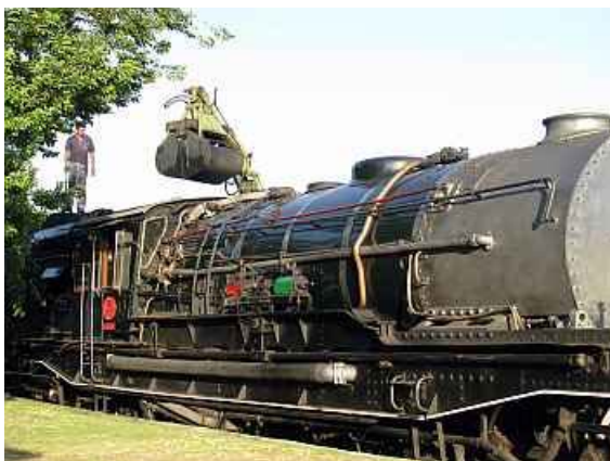
FP01 - Coaling is under way on a hazy Tuesday afternoon. The GMAM is challenging to coal up fully as the coal bunker sides are higher than those of a conventional tender. Because the "Yumbo" coal grab's arms have to be straighter to reach over the high sided bunker, it cannot reach far enough to dump coal neatly on the opposite side - hence the need for a coal trimmer to manually shift the coal over. (PA)
