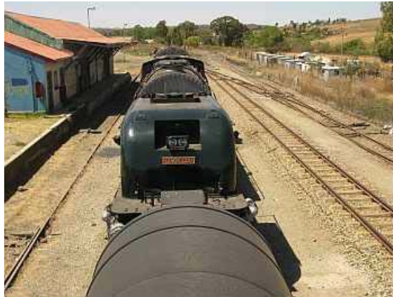
FP36 - A tanker top view of the loco's water tank. The front unit's tank was filled with water as a reserve, but mainly to increase the weight on the front wheels for traction. A problem that standard tank engines face is that they lose adhesive effort as they consume their on-board water and become lighter in weight. The GMA/M series were originally built with facilities to take water from tankers, alleviating the ever lightening weight problem. (LG)
