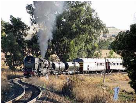
FP49 - With an outlying gold mine dump as a background, this articulated locomotive is about to get some pivoting action going as the train approaches a truly nasty s-bend. This is what Garratts were built for! Notice the mile posts on this section of the line. (PA)
