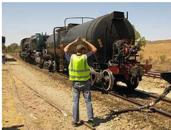
FP38 - Shaun Ackerman is showing the closure signal during the shunting move. You wave your arms slowly like hopeful crab pinchers and show the driver relevant closeness by the resultant space between your hands. When you cross or clasp your hands, the driver brakes and ideally, the diminishing momentum of the moving equipment makes the coupling. A civilized, smooth coupling takes judgement from the shunter as well as the driver. (LG)
