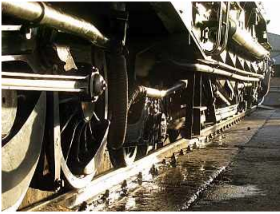
FP05 - An almost mono-chromatic shot of the locomotive at rest over the reception track's ash pit. The reflective spill water is from when the water tank on the front engine unit was filled earlier in the day. (Before the locomotive was turned) Injectors normally puddle a bit, but they are both under slung on the opposite side of this particular locomotive.
