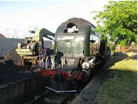
FP19 - Unlike Wilfred's Lyndie Lou., who is a petite, gamine young lady, THIS Lyndie Lou is a hefty girl with a hearty appetite. Not wishing to take chances, the crew put in several extra scoops of coal to top up the bunker once more. Michael Thiel is working on tidying up the just-disconnected water transfer line. A water tanker was on this end, but was dropped off on the Forge House track before coaling. (It turns out the extra coal wasn't necessary.) (LG)
