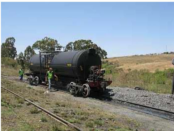
FP31 - Taking the water tanker for a walk. It was pushed up one leg of the turning triangle and left there while the locomotive backed out and preceded up the opposite rails and spotted there. Then the tanker's brakes are unwound and it is rolled down by gravity to be placed behind the locomotive for the homeward bound journey. Shaun Ackerman is walking alongside the handbrake. That equipment on the end deck is our fire fighting pump and hoses (LG)
