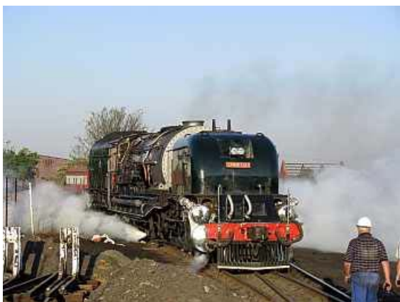
FP03 - Double Blow Down. Duty Shunter Shaun Ackerman takes advantage of the open waste ground next to the forge house for a blow down on the left side, while the opposite valve is still partially open. Note that the blow down drums on the GMAM are under-slung halfway along under the boiler and not astride the throat plate as on conventional locomotives. (PA)
