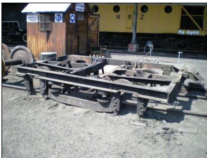
Broken Bogie from Shongololo Express
