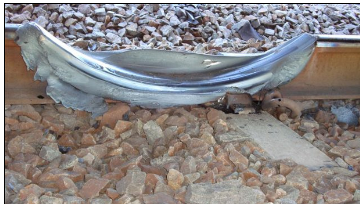
Just to show the power of an Electric Locomotive where an uncontrolled wheel spin had melted a rail.
