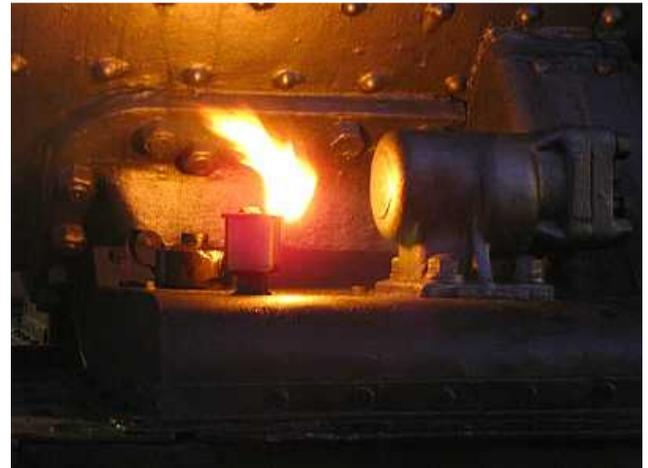
MP03B – The pre-sunrise breeze has picked up and Piet has tucked his guttering flare pot right under the smoke box as a wind shield. The oil pot in the foreground is for the front LHS valve spindle. Luckily the grey graphite paint is heat resistant!
