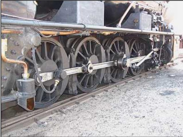
SP01 – Some extra preparation work went into this locomotive! Against the unadorned, solidly black painted goods-train sized wheels (4 feet 3 inches), the newly polished coupling rods and valve gear really stand out. These rods were done with a pneumatic powered flapper wheel but the job is still a long and tedious one with the crannies, recessed webs and gaps needing hand work where the bulky flapper wheel can't go.
