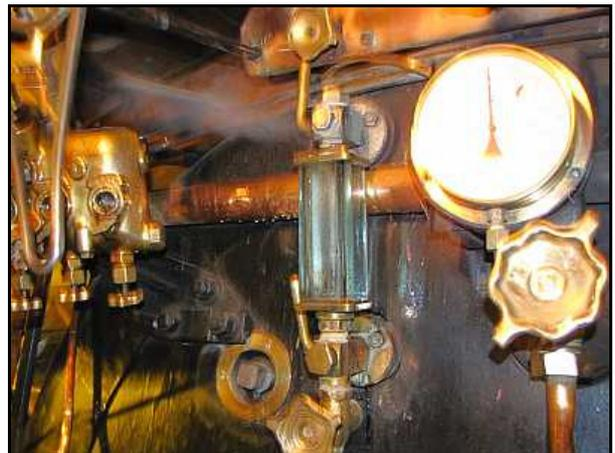
LM06 – The steam test cock on the LHS water column needs repacking. Shutting the test cock off only made the leak worse. The funny thing was that it only showed the ‘steam’ and dribbling water when the water level was higher than the glass – which is what we often do when loco minding. When the water level dropped, the leak was still there – but the escaping steam was invisible and didn’t fog up the inside of the glass. Rather dangerously, it was still capable of scalding the unwary fireman.
