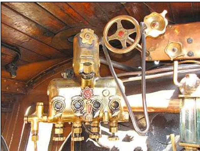
FA03 - The Hydrostatic Lubricator is charged and ready to go – but is bubbling and hissing from the filler plug. The valve with the extension handle is the steam valve for the fireman's injector – this elderly locomotive does not have a Seller's valve set-up, so the steam supply for the injectors is operated directly from the outermost valves on the turrets and not from pull levers from halfway up the left side of the boiler backhead, as with our 15F's, the 25NC and Sandstone's GMAM.
