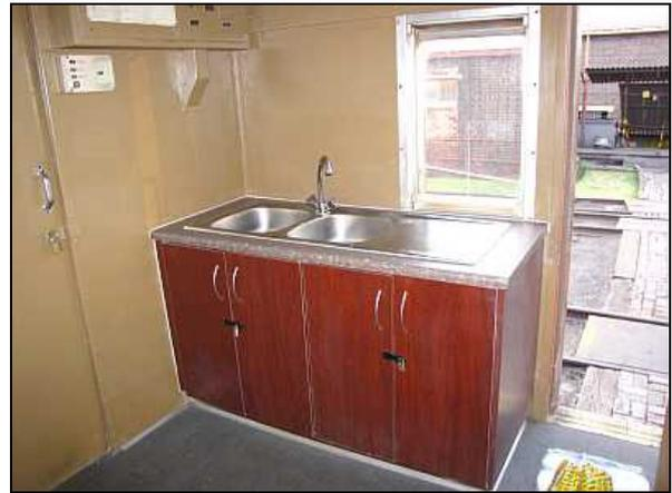
MS01 – Here is a view of the new sink cabinet that has been installed into the old guard's area of the Power Van (ex Staff and Baggage Van) – a matching storage cabinet is out of frame to the left. The Power Van originally had a coupe compartment converted into a kitchen. The old kitchen had been removed and converted into a full shower and washroom facility for the crew. The guard's handbrake still functions – just out of frame to the right.
