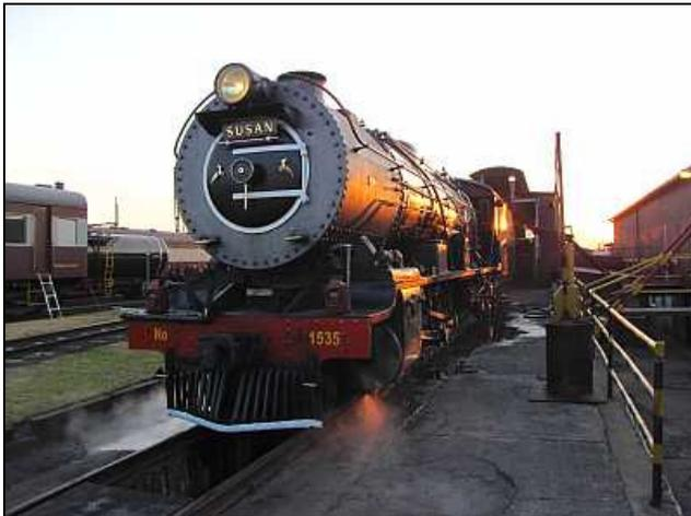
MS04 – A sun-bronzed Susan is just about to be nudged forward to align one of the four holes in the bogie wheels to the 12 o'clock position. This needs to be done to allow access for lubrication of the bogie bearings and the axle horns behind those wheels.
