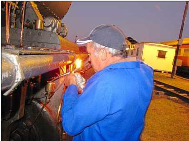
MP03 – Oiling around the engine is usually done after the fire cleaning is done but here it is being done before. Here, in the light of his flare lamp, driver Piet Molentz is topping up the oil cup that lubricates the right-hand-side piston rod. The brass oil cup that feeds oil to the corresponding valve rod can be in line with and to the left of Piet's cap.
