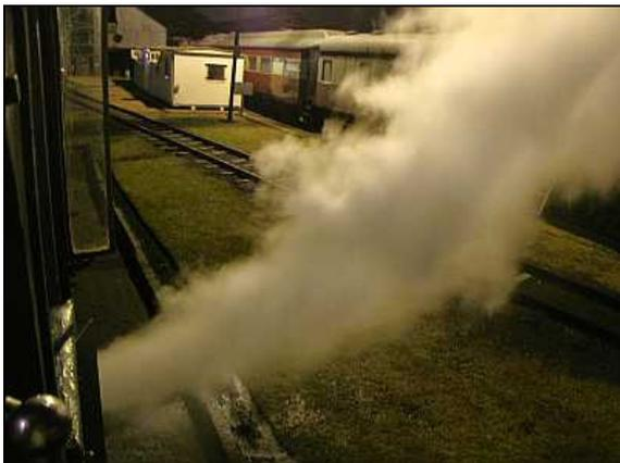
LM01 – A driver's view of a throttled blow-down. The blow down deflector has long since been removed in our recent yard neatening exercises. One needs a bit of restraint if blowing down to manually to reduce the steam pressure from the right hand blow downs when on the reception track. Even so, the adjoining coaches and the water tankers got drenched in condensation.
