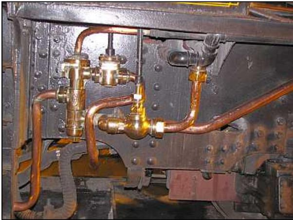
LM03 – Susie’s beautifully polished right-hand-side injector set. Steam is fed from the copper pipe at the top, and the water is fed in through the question mark shaped pipe and through the foot-operated valve. The overflow discharge is through the dogleg pipe off to the left (under the steps) and the pressurized feed water to the boiler is via the diagonal pipe to the right.
