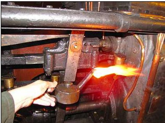
MP04 – While Piet Molentz grumbled away for a top-up of his oil can, I got a close up of the unattended flare lamp with the flame flapping in the freshening morning breeze. It is basically a paraffin lamp with a woven wick in the long spout. Such a lamp looks primitive but usually provides better light than most modern torches and doesn't need to be set and have the beam aimed while the driver's two hands are otherwise engaged.
