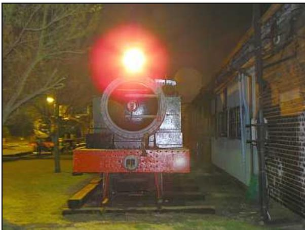
LM05 – Patrys, the plinthed Class A tank engine, now has a working headlight which was wired in to mains power during Fred Sewell’s yard lighting project. (The original Pyle Industries turbine-dynamo is still present above the LHS water tank though.)
