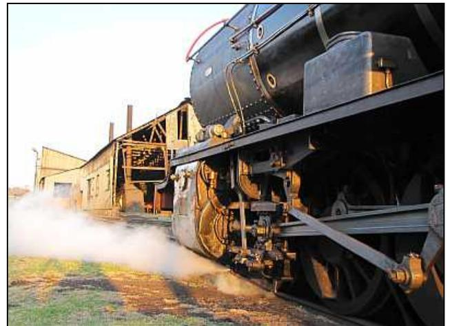
LD02 – The leaking gland pointed out in photo SP04 has since been serviced and we now have a clear view of the rear cylinder head end of the steam chest, helpfully spot-lighted by the early morning sun. The rods still look clean from their polish of two weeks previously.
