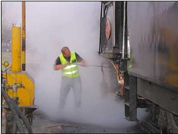
MP06 – Finally it is fire cleaning time and a gently steamed Riaan Coetzee comes to grips with the two pathetically small oval shaped holes which are all that is provided on either side to rake down the ash pan on the Class 12AR. The steam exhaust is from the grate shaker cylinders and the copious discharge has encouraged Riaan to take off his glasses. The fierce, staccato grate shaker exhaust noise is quite hard on the ears too.
