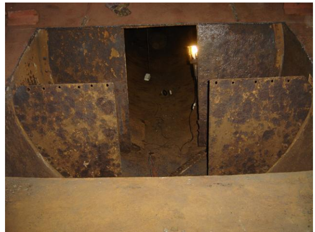
New tender plating in place
