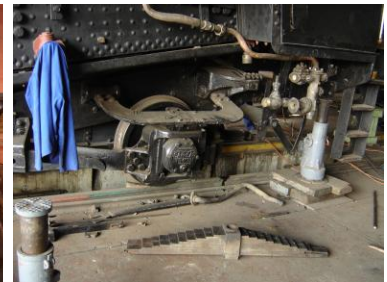
New bissel bogie springs
