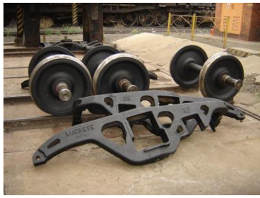
Newly rebuilt tender bogie frames & wheels
