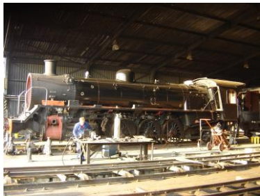
2654 takes shape with new cladding fitted
